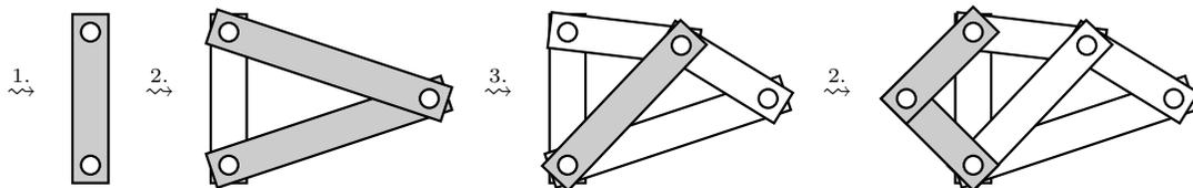
Figure 2: Example construction of a rigid graph. Note that the architect may add additional balks afterwards.
