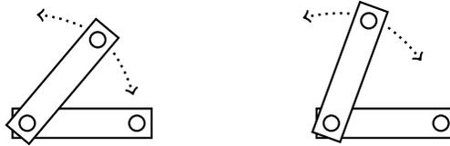
Figure 1: The balks can rotate freely around their connecting axis.
